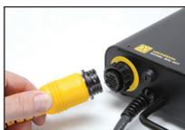
To insert the cable, position the logo up to align the key ways on the extension cable with the circular receptacle on the ballast. Rotate the locking ring until it clicks into the lock position.
