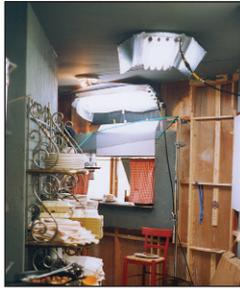
The grommet holes along the edge of the fixture are designed to allow the fixture to be screwed onto set walls.
