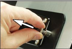
**To remove the plate**, pull up on the locking pin and reverse the mounting procedure.
